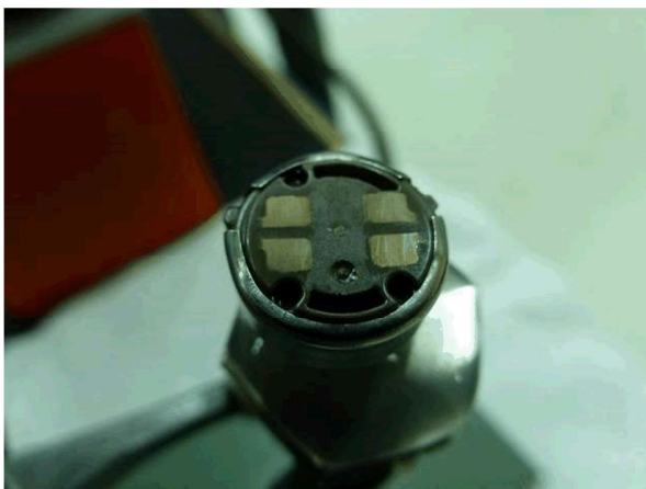
No leakage at contacts of sample 48
