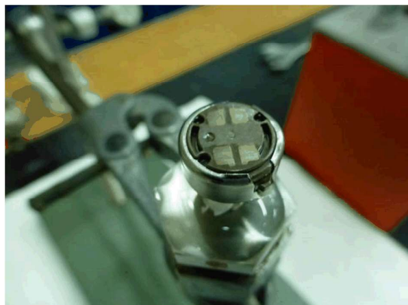
No leakage at contacts of sample 49
