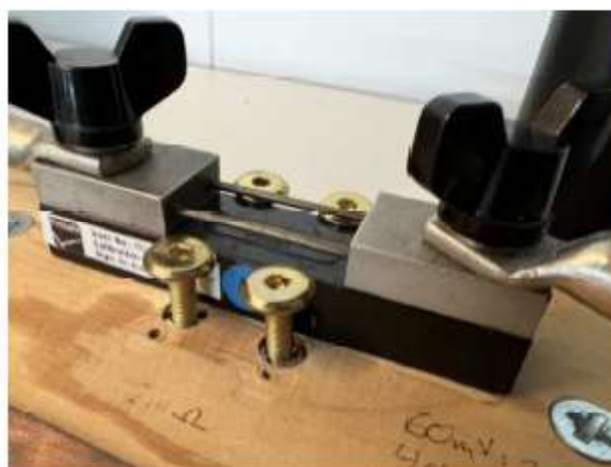
Probe for oscilloscope measures voltage drop over shunt resistor. Short circuit current is then calculated ( I = U / R ).
