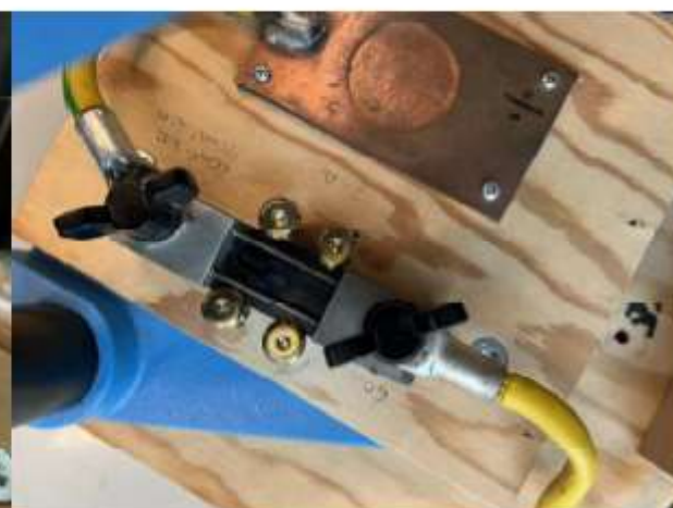
Calibrated shunt resistor of 2mΩ.
