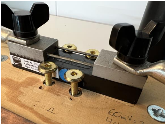
Probe for oscilloscope measures voltage drop over shunt resistor. Short circuit current is then calculated ( I = U / R ).
