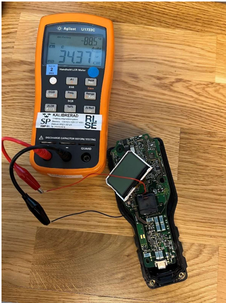
Test 1: Maximum voltage: 18,9V
