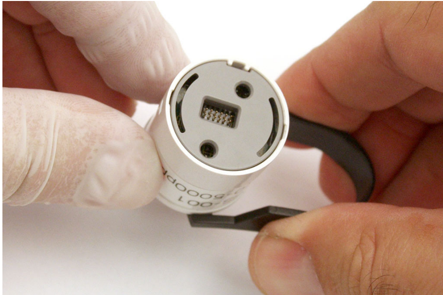
Figure 30: Using Removal Tool
