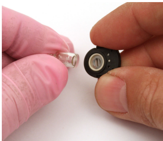
Figure 33: Reinstalling the Electrode Lamp
