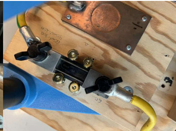
Calibrated shunt resistor of 2mΩ.
