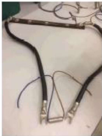
Short circuit current resistor (5 mOhm)
