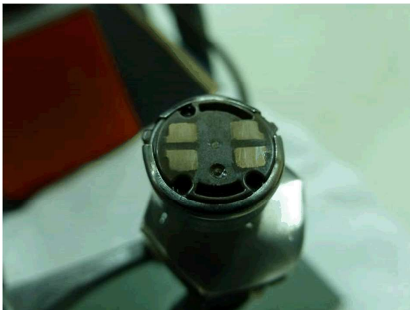
No leakage at contacts of sample 48
