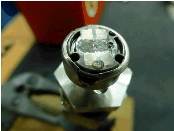
Leakage at contacts of sample 50 > 1200 kPa
