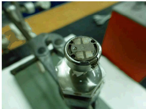
No leakage at contacts of sample 49
