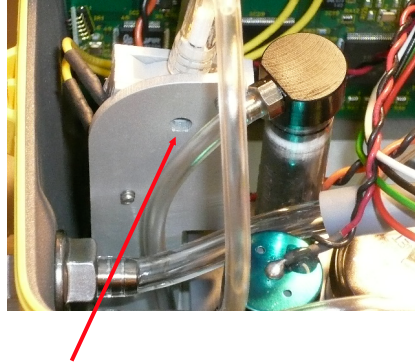
DP switch adjustment screw
