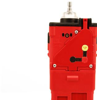
Remove the three screws holding the flow chamber and remove flow chamber from unit.
