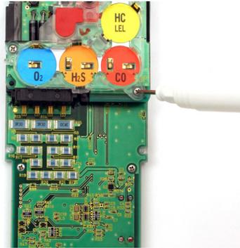
Remove the 3 screws holding in the Sensor board.
